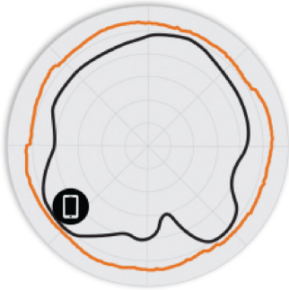
Figure 2. 2.4GHz Azimuth Antenna Patterns
